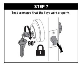
Installation Guide - Exposed Screw Lever
